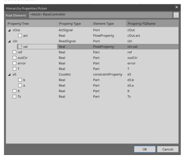
We select property *val* under *cIn* and click on the OK button. The property *val* will be created on the diagram inside the Port *cIn*, and a Binding connector between *cIn.val* and *e6.c* will be created. After binding parameter *e6.a* to property *error*, and *e6.b* to property *ref*, the diagram will resemble this:
