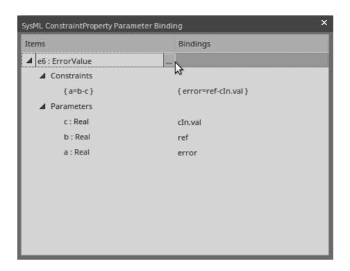
Click on the button on the right to edit the typing Constraint Block. The 'Edit Constraint Block' dialog displays.
