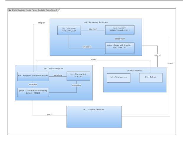
The example describes the Portable Audio Player's composition, detailing how each of the subsystems is structured. The example also describes the binding relationships between the parts, which define how they are functionally bound to one another; for example, the CPU, Memory and Codec are interfaced together in the Processing Subsystem.
