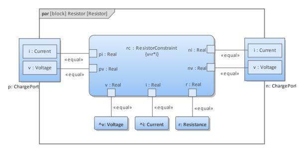
A typical system can contain multiple Parametric diagrams, each defining a specific engineering analysis of specific parts of the system.
