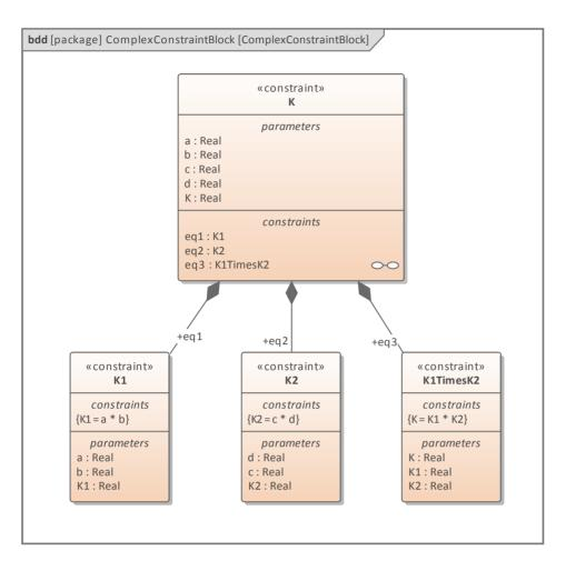
Rather than extract the value of K from one calculation, the system will first calculate K1, then K2, and finally the product of K1 and K2, giving the value of K.
