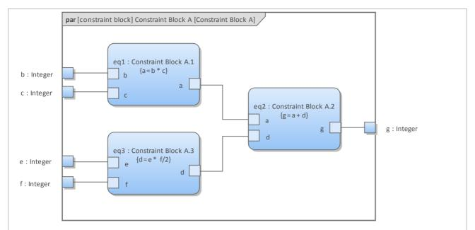
SysML Parametric models support the engineering analysis of critical system parameters, including the evaluation of key metrics such as performance, reliability and other physical characteristics
