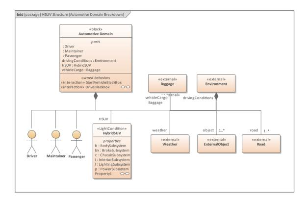
In the example, the Automotive Domain is defined as a system containing other subsystems; the domain contains subsystems that define the Driver (that is, User), the Hybrid SUV, Baggage (which is carried in the vehicle), and the External Environment.
