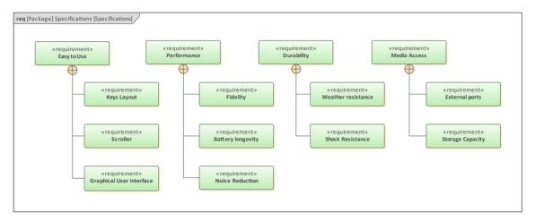
This example displays several top level requirements such as 'Ease of Use' and then breaks those requirements down into more refined requirements such as the 'Graphical User Interface'.
