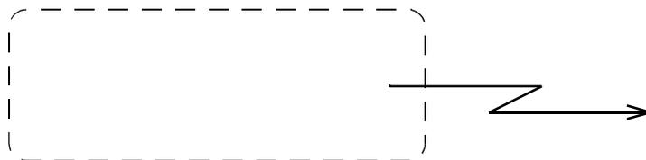
Figure 258 - InterruptibleActivityRegion notation with interrupting edge
