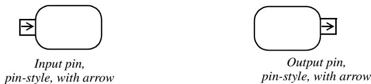
**Figure 284 - Pin notations, with arrows**
