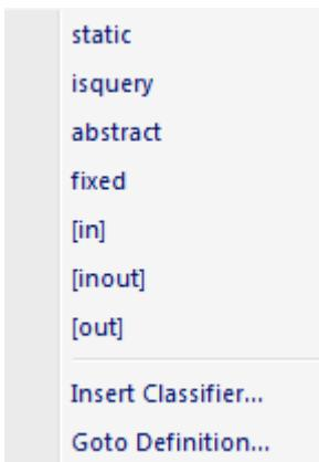
6. Select the appropriate menu option for the parameter kind value: **[in]**, **[inout]** and **[out]**. The diagram is updated to reflect the change.
