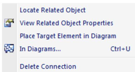
If an element is not present in the current diagram, the context menu contains the **Place Target Element in Diagram** option. This is useful when you are building up a picture of what an element interacts with, especially when reverse engineering an existing code base.
