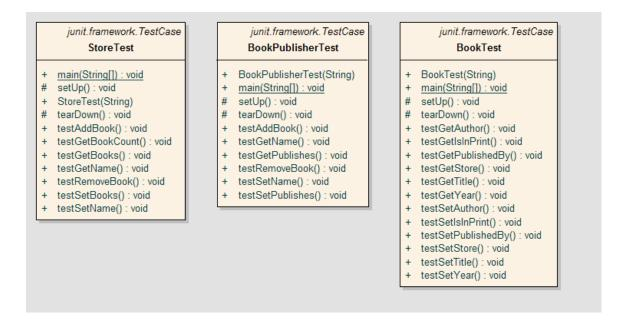
The test code skeletons can now be generated from the resulting classes, edited in an appropriate IDE to add the test logic, and executed after loading them into the JUnit framework.
