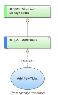
This diagram shows a Use Case that realizes a requirement. The realized requirement is part of a hierarchy of requirements expressed with the Aggregation relationship. The Use Case has an annotation under the element indicating its package location in the Project Browser.
