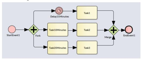
Execute this model and click on 'Generate multiple timelines for each token' the generated Timing diagram resembles this:
