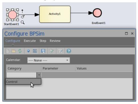
• After the category selection, the combo box in the 'Parameter' column will be filled with all the available parameters for the selected element
