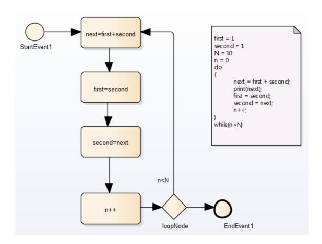
The pseudocode of the process is shown in the Notes element on the diagram. The statement 'print(next)' will output the number series 2, 3, 5, 8, 13, 21, 34, 55, 89, 144. The BPSim configuration for this process is set up as described here.
