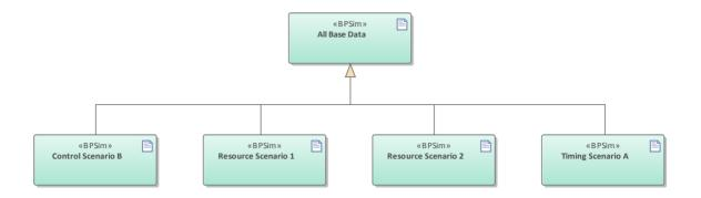
When you run a simulation on a scenario configuration, it will inherit the data defined in the base configuration and the simulation will perform as if it were processing a single configuration containing all the data. If the scenario configuration contains data that is also defined in the base, the (changed) values in the scenario take precedence.
