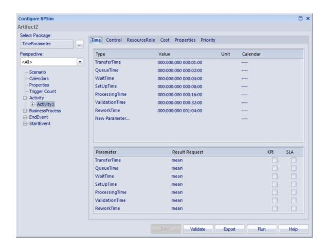
Note that in the upper panel there are seven system-supplied 'Time' parameters, which have been given initial values of - in order - 1, 2, 4, 8, 16, 32 and 64 minutes (the 64 minutes is 1 hour and 4 minutes). Note also that in the lower panel, each of these has a Result Request for the mean runtime value of the parameter.
