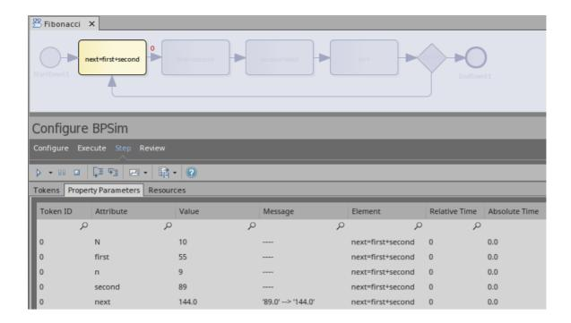
Keep clicking on the Step in button; the properties in the list will change their values. This figure shows that on entering task 'next = first + second', the value of property 'next' changes from 89 to 1<sub>44</sub>.
