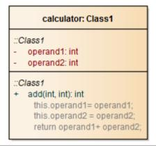
On the simulation diagram, for the appropriate Action element, open the 'Properties' dialog and on the 'Effect' page type in the JavaScript to capture and simulate the Object's behavior.
