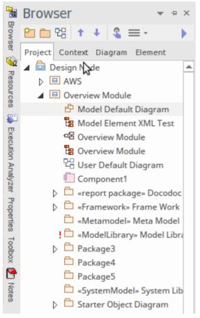
When you move the cursor over the tab, the window overlays the screen and you can work within it. As soon as you move the cursor out of the window, it automatically contracts into the margin tab again. This means that you have the maximum work area for performing your main task, with the convenience of still being able to immediately use any of a wide range of other windows.
