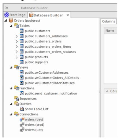
In this image the data model 'Orders (postgres)' shows logical folders for Tables, Views, Functions, Sequences, Queries and Connections. It is worth noting there is no folder for 'Procedures' since PostgreSQL does not support database procedures.
