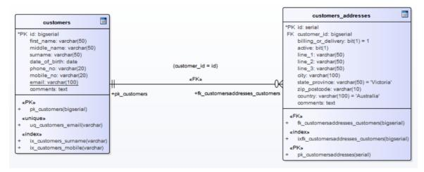
Each Table defines database columns, using UML attributes typed appropriately for the target DBMS (in this case, PostgreSQL).
