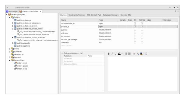
This figure shows the Database Builder loaded with the 'Orders (postgres)' data model as it appears in the Example model
