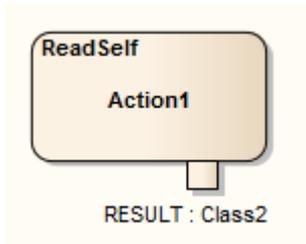
The Action must be within a Class, which is instanced during run time. When a simulation passes the Action, it puts the name of the instance of the Class into the result Port.
