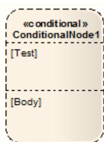
You define Conditional Nodes by dragging other Activity diagram elements from the Toolbox page into the appropriate partition of the element, and linking and organizing the structure as required. The elements are
