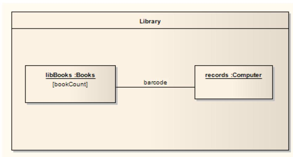
In this diagram there are two Parts, 'libBooks' and 'records', which are instances corresponding to the Classes 'Books' and 'Computer' respectively. The relationship between the two Parts is indicated by the connector, reflecting that communication between the Parts is via the barcode. This contained structure and its Parts are properties owned by the Library Class.
