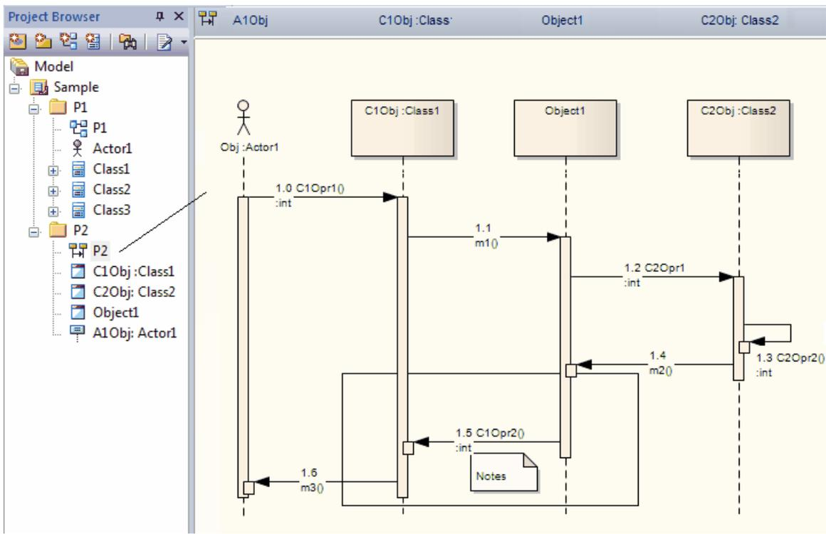
This diagram is not damaged, because all the Lifelines are objects and these objects reside in the same Package as the Sequence diagram.
