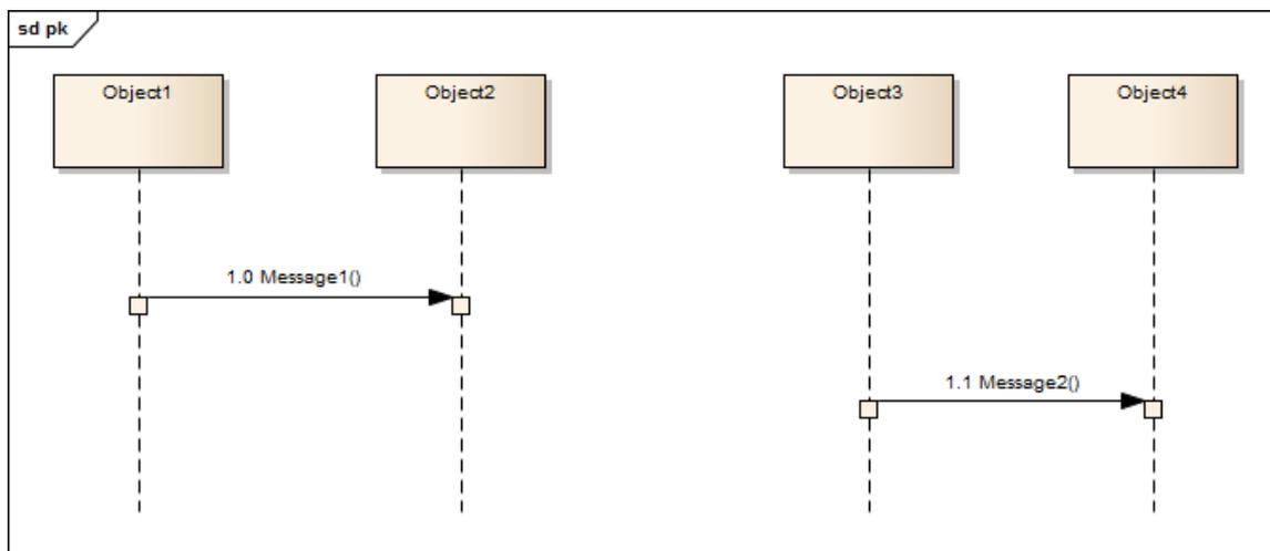
In the diagram, Message 1 is earlier than Message 2. However, in a complex diagram, or when representing finely timed operations or parallel processing, this might not be apparent. You can reinforce the sequence using a 'General Ordering' arrow.
