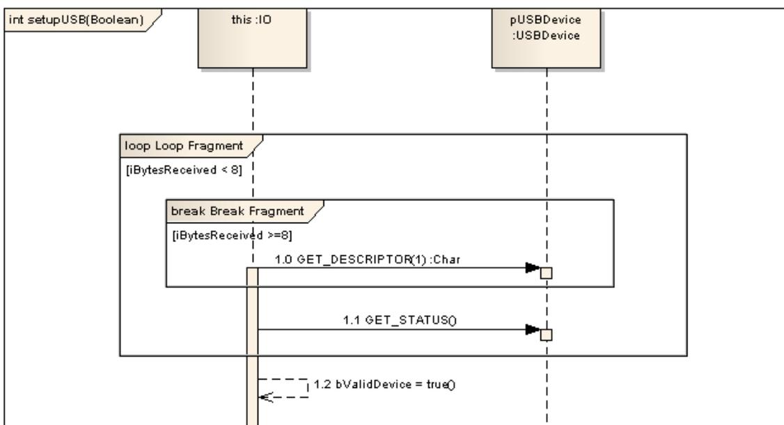
An Interaction element in Enterprise Architect is treated as a behavior of the classifier it is encapsulated within. It can have parameters and return types, which are modeled using
