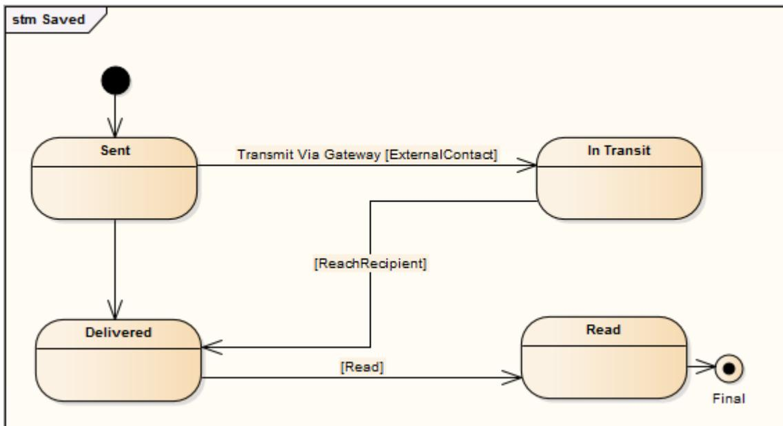
By default, the child diagram displays within a labeled frame that represents the parent object in the context of the child diagram. You can right-click on the background and select the 'Hide Diagram Frame' option to hide the frame, and on the 'Show Diagram Frame' option to show the frame again.
