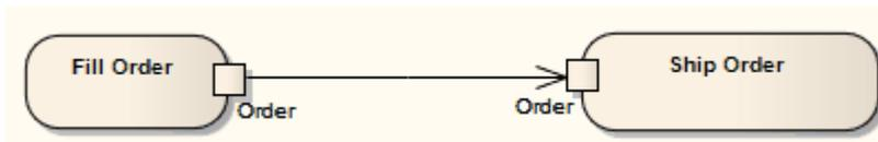
Action Pins can be further characterized as defining exception parameters, streams, or states. Associating a state with a Pin defines the state of input or output values. For instance, the Pin could be called 'Orders', but the state could be 'Validated' or 'Canceled'.
