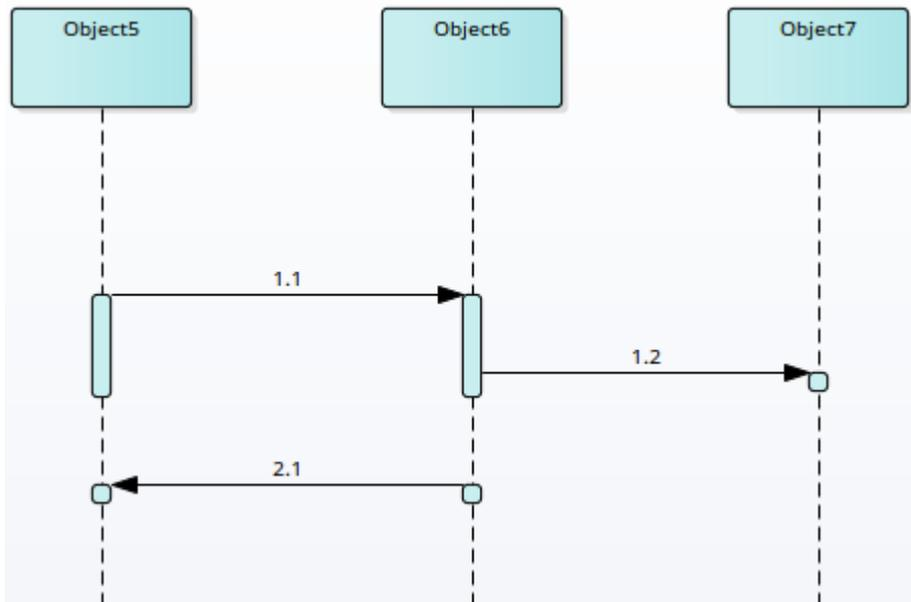
Message 1.1 passes from Object 5 to Object 6, and then Message 1.2 passes to Object 7 and Message 2.1 passes back to Object 5. It appears that the Messages go in the sequence 1.1, 1.2 and then 2.1. However, you want to indicate that Message 2.1, whilst separate, is concurrent with Message 1.2.
