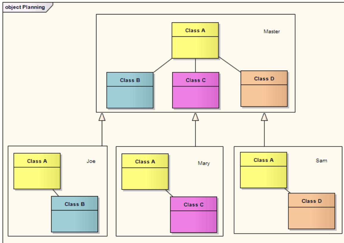
A Diagram Frame element is a rendition of a diagram dropped from the Browser window into another diagram. It is a type of Combined Fragment with an 'Interaction Operator' ref. However, it can be created on any type of diagram, and is not created in the same way as other Combined Fragments.
