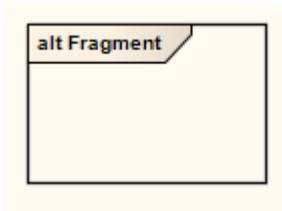
A Combined Fragment reflects one or more aspects of interaction (called interaction operands) controlled by an interaction operator, with corresponding boolean conditions known as interaction constraints. The Fragment displays as a transparent window, divided by horizontal lines for each operand.
