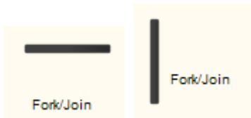
The Join element is used by Activity and StateMachine diagrams. The example illustrates a Join transition between Activities. With respect to StateMachine diagrams, a Join pseudostate indicates multiple States concurrently transitioning into the Join and onto a single State. Unlike Choice or Junction pseudostates, Joins must not have triggers or guards. This diagram demonstrates a Fork pseudostate dividing into two concurrent Regions, which then return to the End State via the Join.
