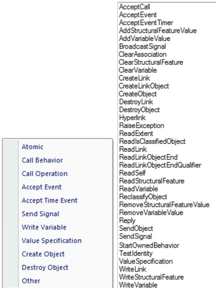
If you later decide that the Action type is not appropriate, you can change it on the 'Action' tab of the Properties window - select the required new type from the 'Kind' drop-down list. For a Value Specification Action, you can also set the value on this tab.
