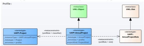
In the Profile example, a Meta-Constraint connector is drawn from the stereotype ActualProject to ActualProjectRole and the constraint is specified as 'slot' on the tag 'umlRole' in the connector's Tagged
