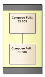
Composed diagrams are currently only supported as the center sub-shape of the main shape. Adding the diagram to any other location will cause the composed diagram to either not draw correctly or not draw at all. The diagram can be a sub-shape of a sub-shape, but only if the parent shape and sub-shape(s) all have a "CENTER" orientation. For example:
