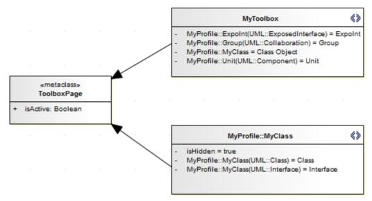
When this Profile is in use, and when the Class Object item is dragged onto a diagram from the Toolbox, the hidden menu displays giving the choice of Class or Interface; on selection, the element is dropped onto the diagram.
