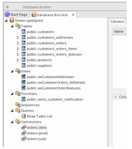
In this image the data model 'Orders (postgres)' shows logical folders for Tables, Views, Functions, Sequences, Queries and Connections. It is worth noting there is no folder for 'Procedures' since PostgreSQL does not support database procedures.
