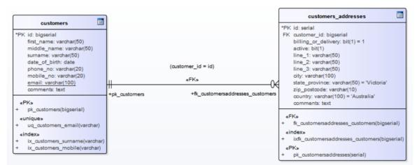
Each Table defines database columns, using UML attributes typed appropriately for the target DBMS (in this case, PostgreSQL).
