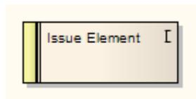
You can link Issues to model elements that are responsible for the issue, using Realize connectors. You can also create a hierarchy of related Issues using Aggregation connectors. Each Issue element has a status band at the left end, which is color coded to visually represent the value of the 'Status' field in the element properties. The element has an identifying 'I' in the top right corner, which you can hide if you prefer not to show it.
