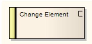
You can link Changes to model elements that are impacted by the change, using Realize connectors. You can also create a hierarchy of related Changes using Aggregation connectors. Each Change element has a status band at the left end, which is color coded to visually represent the value of the Status field in the element properties. The element has an identifying C in the top right corner, which you can hide if you prefer not to show it.
