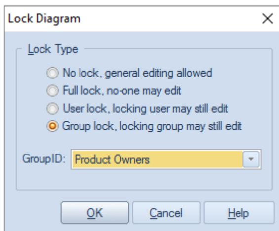
When the Backlog diagram has been locked by the Product Owner, other team members will be able to view the diagram but a small red marker to the left of the diagram name in the Browser window will indicate that it is locked. The Project Manager will see a blue marker indicating that they have access to edit the diagram.
