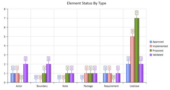
You define this appearance - or its alternatives - on the 'Appearance' page of the element 'Properties' dialog, after having set the 'Type' field on the 'Source' page to 2D Bar. Each change in setting is immediately illustrated by an example Chart on the 'Appearance' page.
