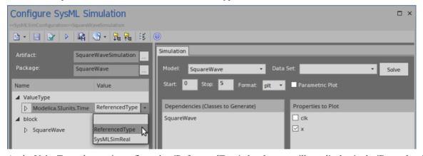
As the ValueType element is configured as 'ReferencedType', the element will not display in the 'Dependencies' list and will not be generated as a new Class definition to the Modelica file.
