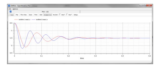
• Mass, light vs heavy: the object with smaller mass will oscillate faster and regulate quicker
