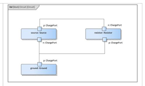
Notice that this follows the same structure as the original circuit diagram, but the symbols for each component have been replaced with properties typed by the Blocks we have defined.
