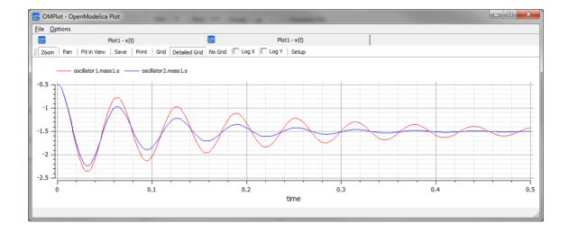
• Damper, no vs yes: the oscillator never stops without a damper
