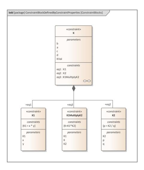
Create a Parametric diagram in Constraint Block 'K' and connect the parameters to the constraint properties with Binding connectors, as shown:
