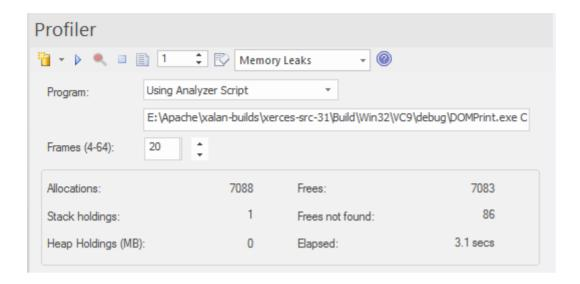
The Profiler control, showing the count of memory allocations and the count of operations that are memory free.
