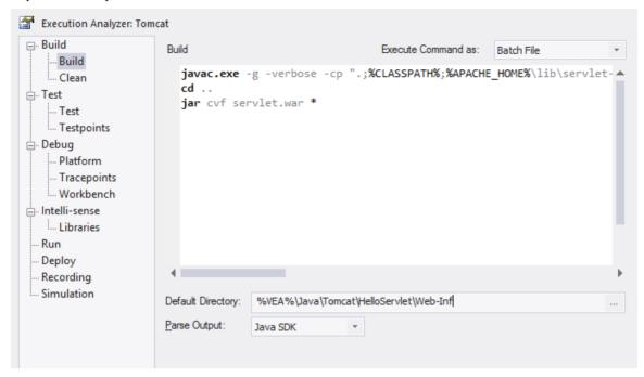
A single project can have multiple configurations and these can be found grouped together in the Analyzer window.
