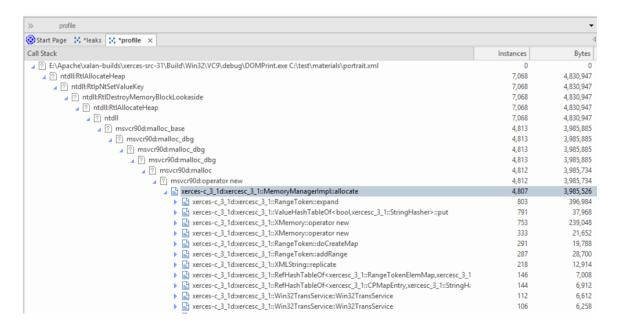
This example is of a report produced from Profiling a demonstration program in the Xerces project from Apache. The program iterates over the Document Object Model (DOM) for a provided XML file.
