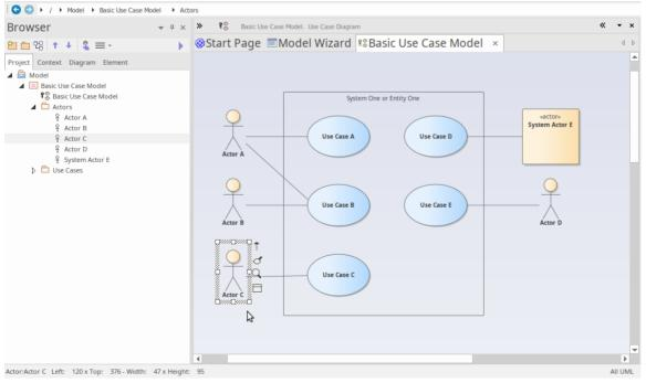
As you can see, there is an underlying model-level element in the Browser window that has a graphical representation in a diagram. Note that you can place a single model element in as many diagrams as you like, and that changing the name
