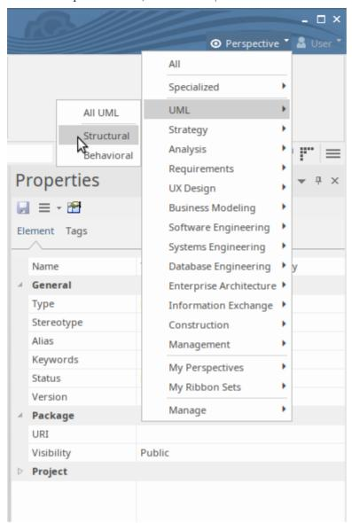
The Model Wizard is displayed, showing the Structural Perspective. Scroll through the list to find the Class diagrams, then click on 'Basic Class Diagram with Operations'. Click the folder icon beside the 'Add To:' field and choose the Model root node as the location in which to add the new model content. Finally, click on the Create Pattern button to add the new model content to your project.
