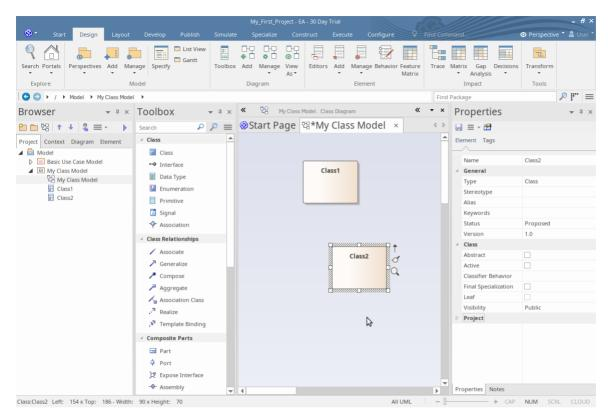
To create a relationship between two elements on a diagram, simply select a relationship type in the Diagram Toolbox, then drag a line from one element on the diagram to another. Most relationships are directional, so dragging a link from Class1 to Class2 is different to dragging a link from Class2 to Class1.
