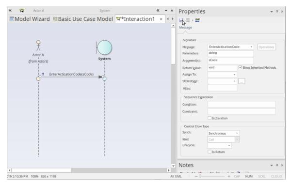
A return message can be created in similar fashion, by clicking on System, then dragging its Quicklink button across to the Actor A Lifeline. Select the new message on the diagram and fill in the details in the Connector Properties window. In the 'Control Flow Type' section of the Properties window, select the option 'Is Return'. Your diagram should now display the return message, similar to this image:
