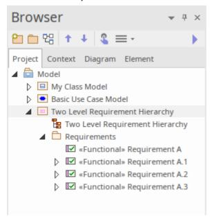
Double-click on the diagram link in the 'Project' tab of the Browser window to open the diagram in the main diagram workspace. You can then select elements on the diagram (or in the 'Project' tab) and use the Properties window to tailor them to your own use, by renaming them, entering descriptions in the Notes window or setting other properties as required.
