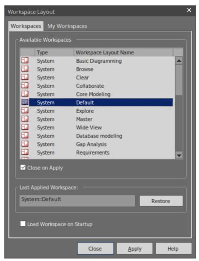
Before you try out some layouts, clear the 'Close on Apply' checkbox, so that you can try different layouts without having to re-open the dialog. Select a layout (such as 'Debug') and click on the Apply button.
