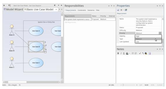
2. Secondly there is the Constraints tab. This tab lets you enter restrictions and constraints on an element's behavior,
