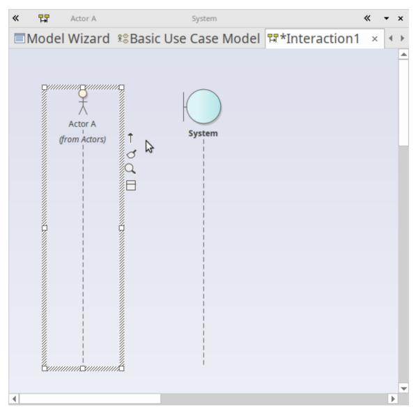
Now, click-and-hold on the Quicklink button, then drag across to the System Lifeline and release. This creates a new message in our model, between Actor A and System. Select the new message on the diagram and note that the Properties window updates to show the properties of the new connector, allowing you to edit the details. After entering a few details for the message and clicking the Save button, your diagram workspace should resemble this image:
