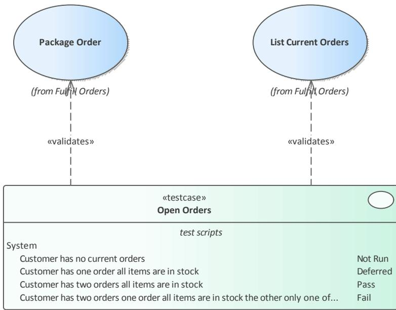
Example of a Test Case validating Use Cases, in Sparx Systems Enterprise Architect.
