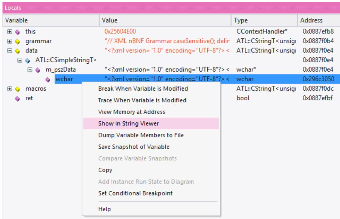
This example shows the value of a variable holding the contents of an XML schema file.
