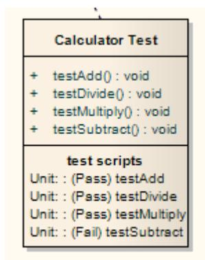
The error description for each failed test is added to any existing results for that Test Case, along with the current date and time.
