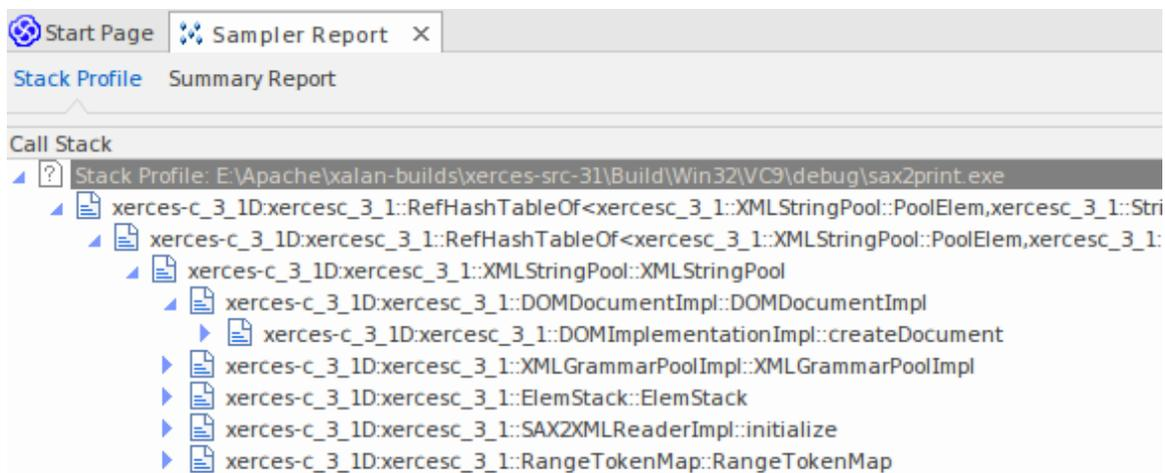
Stack Profiles are taken to discover the different ways (stacks) and the count of ways that a particular function is invoked during the running of the program. Unlike other profiler modes, this profile is activated through the use of a Profile Point, which is a special kind of breakpoint marker. The marker is set in the source code like any other breakpoint. When the breakpoint is encountered by the program, the stack is captured. When you later produce the
