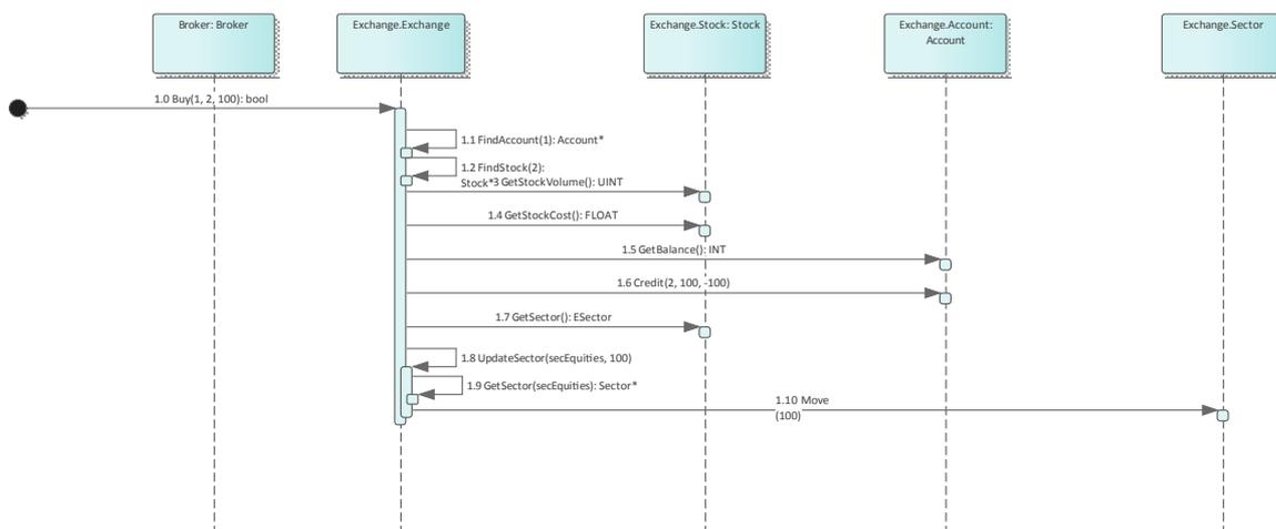
Sequence diagram generated in Enterprise Architect using recording marker in a Use Case
