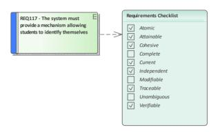
This diagram shows the use of a Requirements Checklist that acts as an indicator (check) to ensure the requirement is compliant with best practice. The check items are editable and a general checklist element is available that can be used with any element.
