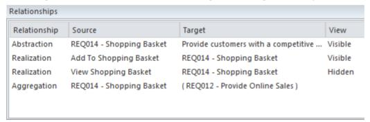
If relationships have been hidden in a diagram they can be made visible by selecting the 'Show Relationships' option on the 'Connectors' page of the 'Properties' dialog for the diagram.
