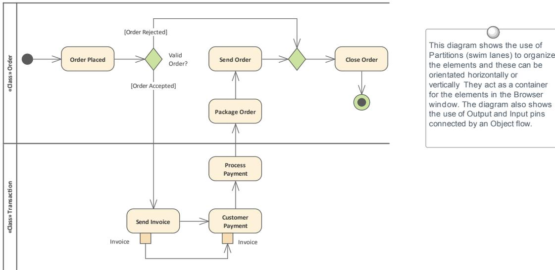
This diagram shows the use of Partitions (swim lanes) to organize the elements and these can be orientated horizontally or vertically. They act as a container for the elements in the Browser window. The diagram also shows the use of Output and Input pins connected by an Object flow.
