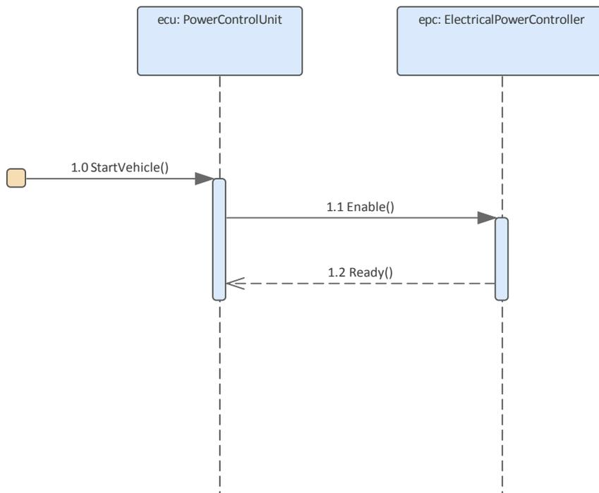
In the second diagram we see a simple Sequence diagram that represents the sequence of messages involved in starting a vehicle. It can be seen from the diagram that there are two Blocks (Instances) that form part of the interaction, and messages are exchanged between the two Blocks and the initiator of the interaction, and ultimately the Use Case.
