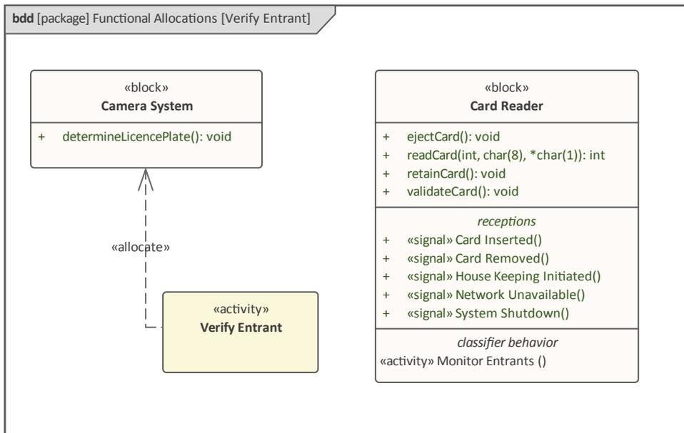
In this diagram the engineer has created two functional allocation relationships that describe how the work specified in the Activity *Verify Entrant* will be carried out. One relationship targets the Camera System that is used to capture the vehicle's licence plate in order to determine if the particular vehicle has been authorized for entry. The other relationship targets the Card Reader Block that is used to determine that the card owner has a relationship with the Parking Station.
