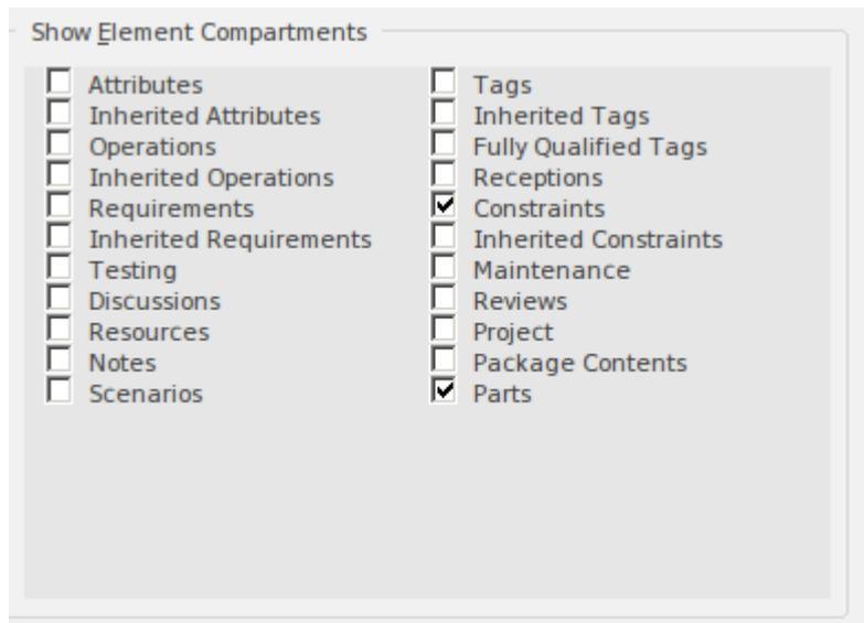
The repository elements will be updated regardless of whether they are edited in the diagram or the Browser or any other window. In the example, the engineer created the Parts in the diagram by dragging a Part Association from the Toolbox; in response to this Enterprise Architect creates three new Parts, which are placed under the Chassis node in the Browser as indicated in this screen shot.
