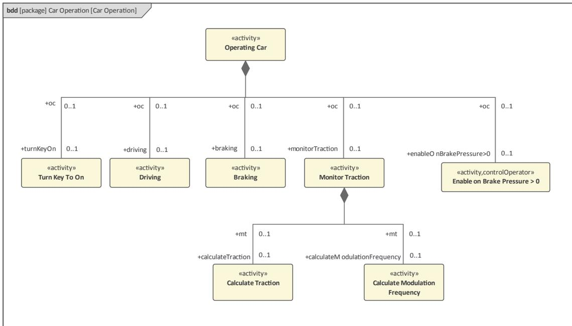
In this diagram a break-down structure has been used where an activity is decomposed into a number of more granular activities using the Composition relationship. There are a number of relationships which have been grouped together to make the diagram more appealing, using one of the flexible line styles available from the diagram context menu.
