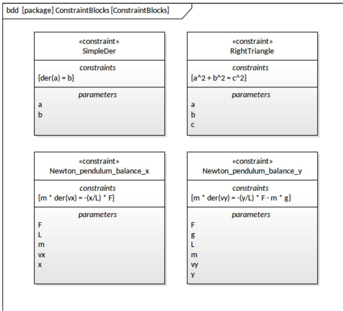
The next step is to create the Parametric diagrams that bind the equations together. As discussed earlier in the Guide, these diagrams are a specialized type of Internal Block diagram and contain instances of ConstraintBlocks called ConstraintProperties that expose their parameters, which are bound by connectors to parameters on other ConstraintProperties.
