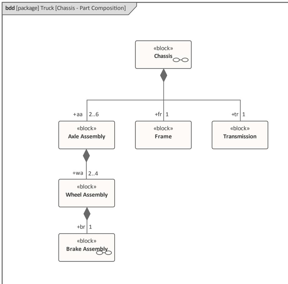
In the diagram the modeler has expressly defined the Parts by using the Part Association, available from the **SysML Block Definition** toolbox.
