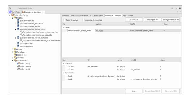
In the image there is only one Table that had detected differences - 'public.customers\_order\_items'; selecting this populates the 'Components' list. From the detected results it can be determined that the data model contains a column (tax\_amount2) and a check constraint (ck\_customerordersitems\_discount1) that the live database doesn't and in turn the live database contains a column (tax\_amount) and a check constraint (ck\_customerordersitems\_discount) that the data model doesn't.
