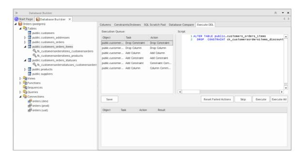
In summary, DDL is generated to drop both the old column and the old constraint (tasks 'Drop Column' and 'Drop Constraint'), then the column and constraint are created with the new names (tasks 'Add Column' and 'Add Constraint') and finally each has their comments/remarks applied (tasks 'Add Constraint - Constraint Comment' and 'Add Column - Column Comment').
