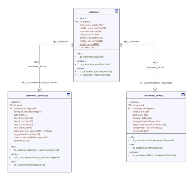
Physical Data model showing Tables with Columns and Primary and Foreign Keys.
