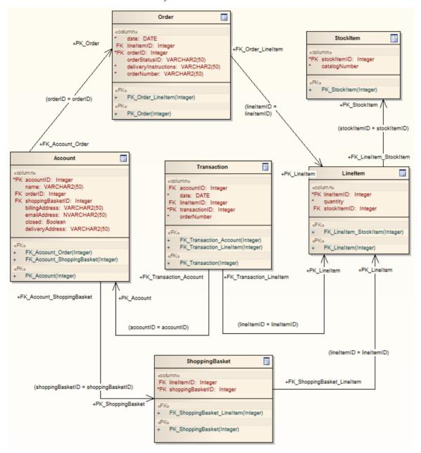
Generalizations are handled by providing the child element with a Foreign Key to the parent element, as shown. Copy-down inheritance is not supported.
