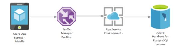
Diagram showing an mobile application using a Smart Phone< traffic Manager and PostgreSQL Database
