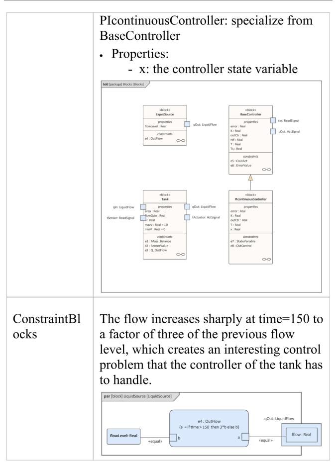
The central equation regulating the behavior of the tank is the *mass balance* equation.
