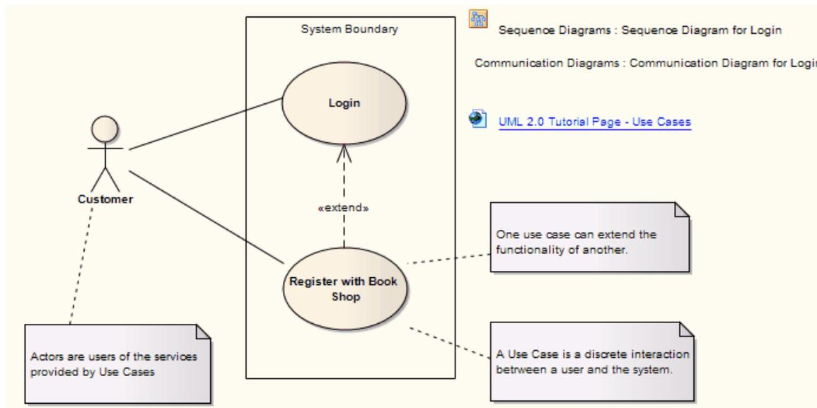
If extending a Use Case, you can specify the points of extension with Use Case Extension Points. To display the attributes, operations or constraints of a Use Case on a diagram, use Rectangle Notation.
