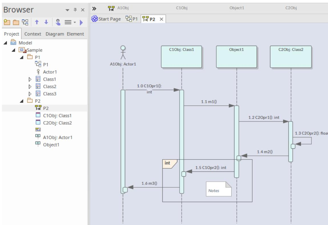
This diagram is not damaged when round-tripped through Version Control, because all the Lifelines are objects and these objects reside in the same Package as the Sequence diagram.
