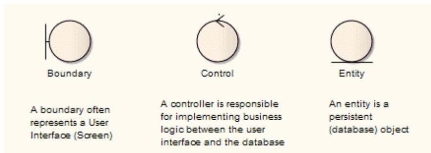
You apply a new appearance or shape by associating the stereotype with either a metafile (image file) and fill, border and text colors, or a Shape Script that defines the shape, dimensions and text of the object.
