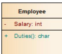
Class elements are generally used in Class diagrams and **Composite Structure** diagrams.
