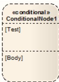
You define Conditional Nodes by dragging other Activity diagram elements from the Toolbox page into the appropriate partition of the element, and linking and organizing the structure as required. The elements are aligned on the top left of the partition, so that resizing the node maintains the organization of the structure within and between the partitions. If you try to shrink the node below the structure size, the node automatically defaults to the 'best fit' size.
