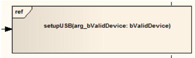
An Interaction Occurrence (or InteractionUse) is a reference to an existing Interaction (Sequence) diagram. Interaction Occurrences are visually represented by a frame, with 'ref' in the frame's title space. The diagram name is indicated in the frame contents.
