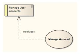
The more usual realization relationship is between a Requirement and a Use Case. A Requirement can be realized by one or more Use Cases, and a Use Case can realize one or more Requirements. Whilst a Requirement defines a condition that must be met, the Use Case is the key to defining and visualizing how that condition is met. A Use Case diagram depicts the logical grouping of actions, processes and components to achieve a
