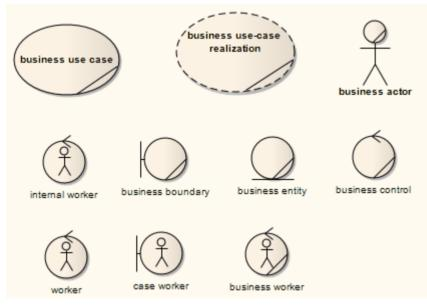
This diagram shows the appearance of the elements dragged from the 'Business Modeling' pages of the Diagram Toolbox and dropped onto a Business Interaction diagram.
