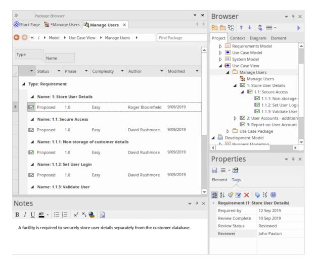
This display shows the position of the Store User Details Requirement element in the model, and how it relates to other Requirements (Browser window); the default characteristics of the Requirement (Package Browser) and the extended characteristics ('Tags' tab of the Properties window), and a detailed description of the Requirement (Notes window). You can configure some of these windows to display more information, and/or use other windows and facilities.
