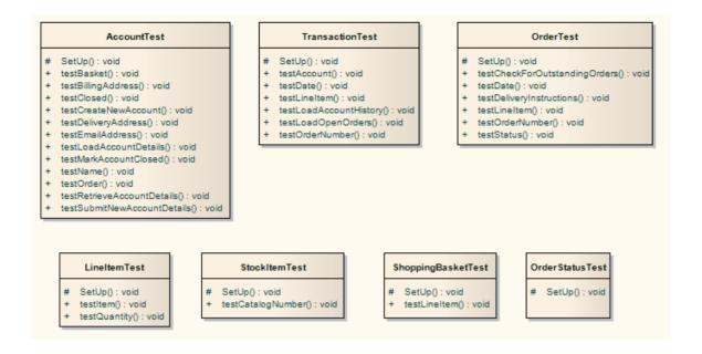
• For each Class in the C# model, a corresponding Test Class has been created containing a test method for every public method in the source Class, plus the methods required to appropriately set up the tests; you fill in the details of each test
