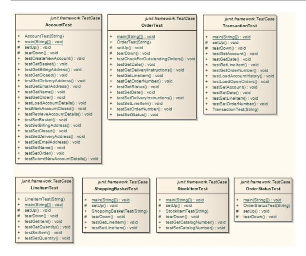
For each Class in the Java model, a corresponding Test Class has been created containing a test method for every public method in the source Class, plus the methods required to appropriately set up the tests; you fill in the details of each test
