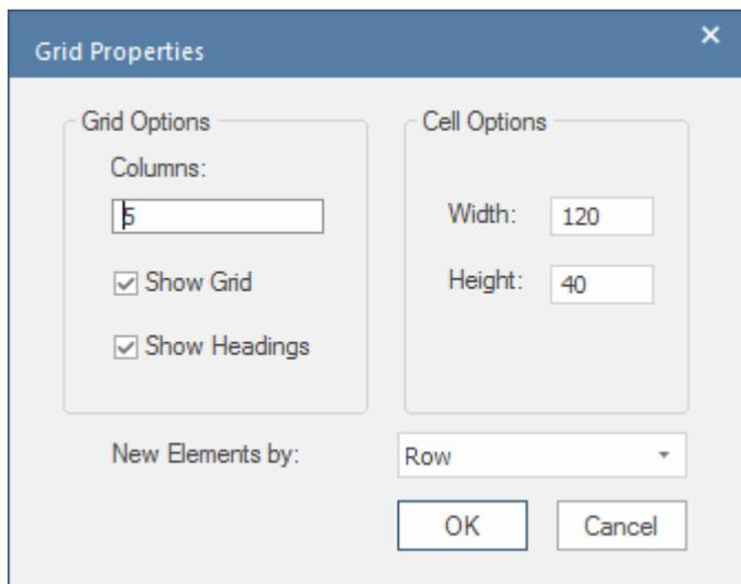
The dialog can also be displayed at any time after grid-style has been enabled, by selecting the context menu option 'Grid > Edit Grid'.
