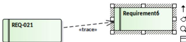
The connectors and elements listed on the two menus depend on the type of the element you initially selected; for example, if you click on the Quick Linker arrow for a Class, the options are not the same as if you clicked on the arrow for an Actor. However, in either case the menus show the most appropriate, commonly used connectors and target elements for that initial element; you can create other connectors and target elements by selecting them from the appropriate Toolbox page.
