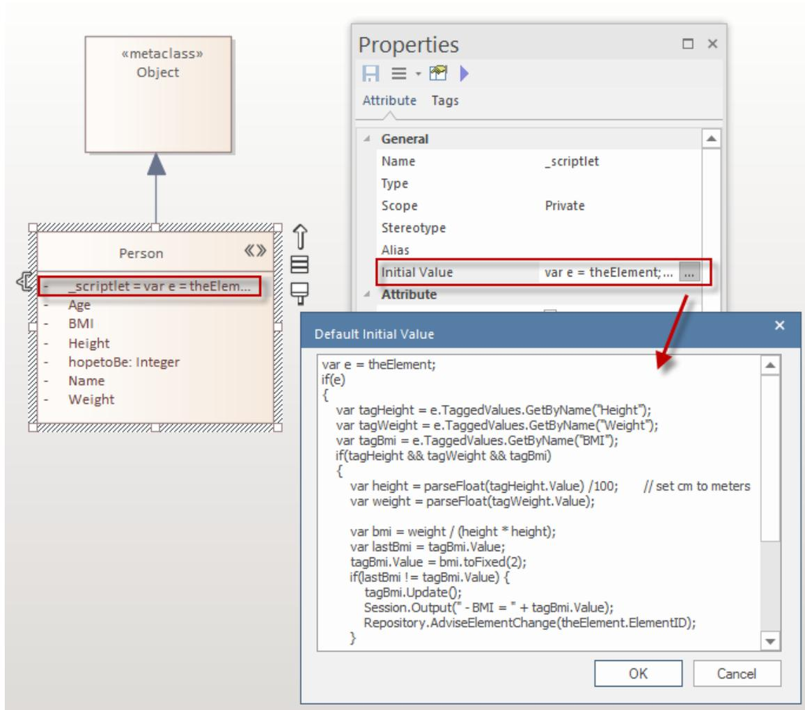
Here is an example of an element created using the 'Person' stereotype, that includes the BMI Scriptlet.
