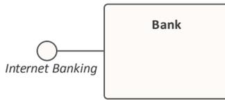
To depict the interfaces that a Class realizes as nodes, right-click on the Class and select 'Features | Show Realized Interfaces'. This setting only applies to the selected Class, and can be changed at any time. If you turn the option off, in the scenario here, neither the node nor the Interface element are shown. If you turn the option back on, the node redisplay.
