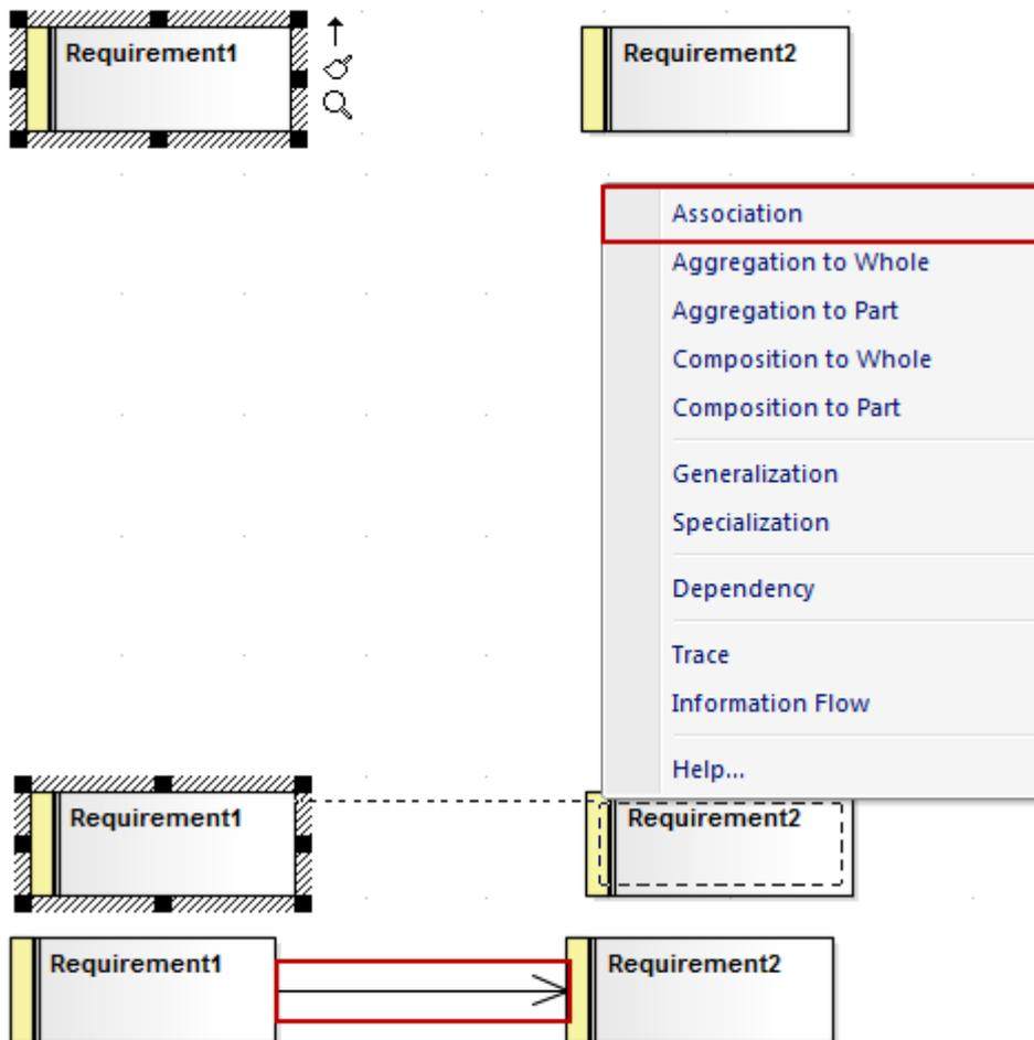
The connector list does not actually display until you release the mouse button over the target element; however, a dotted line shows where the connector would be at any point, and a hatched outline displays within the border of an element as you move the cursor onto it - this helps you identify where the connector should connect to, if there are many closely-arranged elements, Parts, Ports or other extensions.
