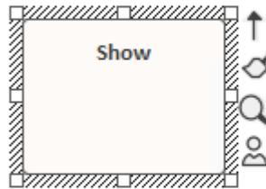
Click on this arrow and drag it in the direction in which you want to create the new connector and element. When you release the mouse button, the element menu displays. When you select an element type, the connector menu displays.
