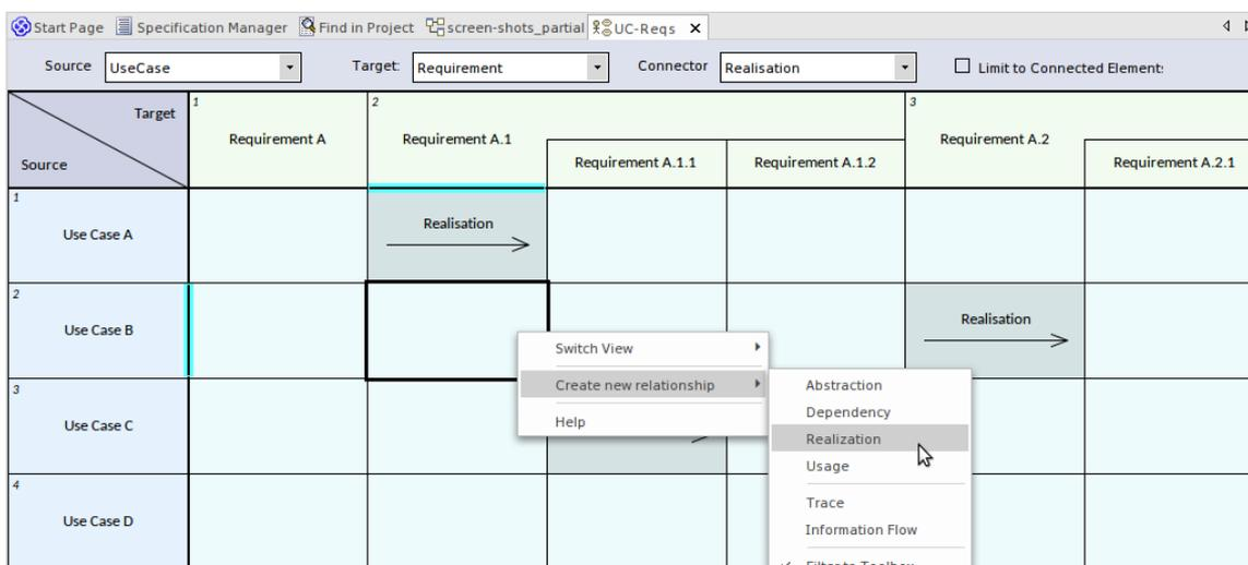
The Relation Matrix view provides a means to quickly identify elements that are not yet connected to other elements, such as Requirements elements that are not yet realized. You can also create new relationships or delete existing relationships directly in the matrix.
