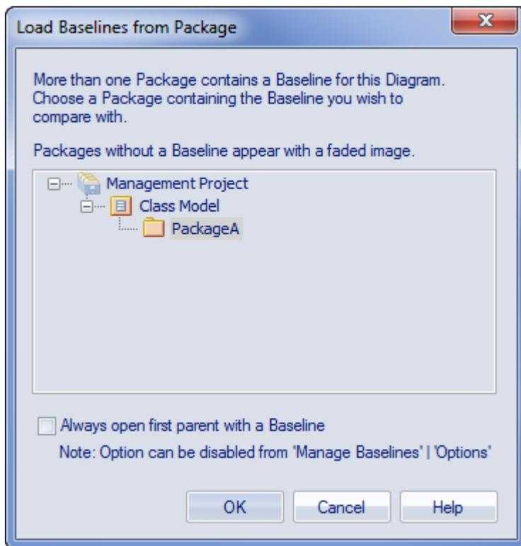
The 'Load Baselines from Package' dialog provides the facility to compare the diagram with one of a broader range of Baselines than just those from the diagram's immediate parent.
