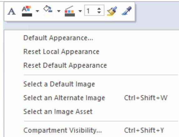
The toolbar icons, in order of display, enable you to set the element's text font, text color, fill color, border color, and border line width, or to set the element fill color to a previously-sampled color, or to sample (copy and store) the current element fill color.
