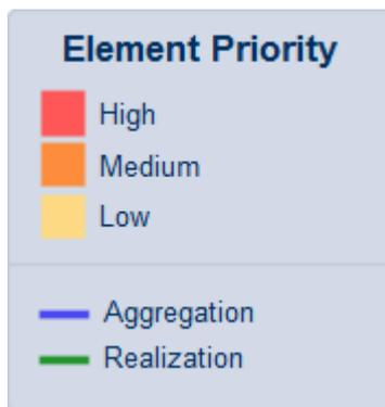
You work on a Legend element in two stages: first create and define the Legend element itself, then define the appearance styles as displayed on the diagram.
