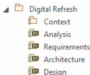
Browser window showing one Checked-Out Package (Context) and four Checked-In Packages under Version Control.
