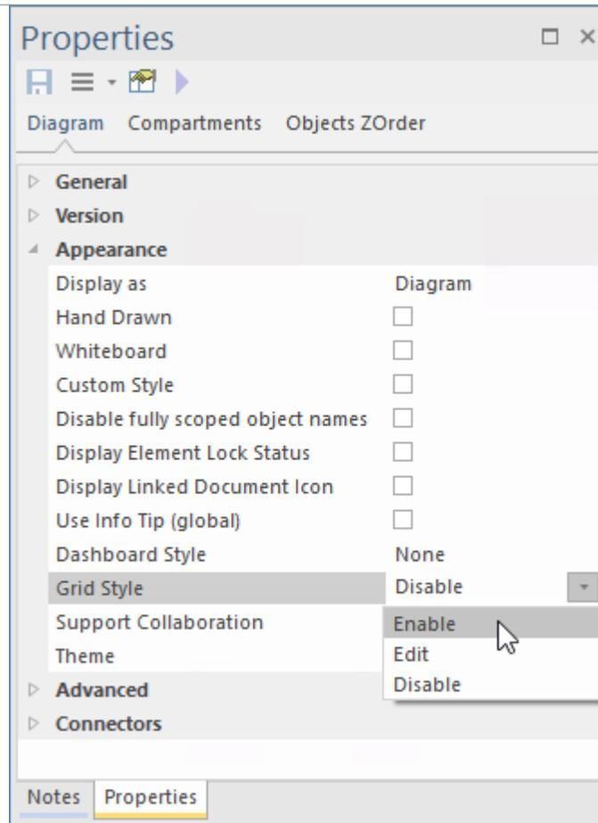
This action turns on the 'grid-style' setting and opens the 'Grid Properties' dialog, where you can specify the Grid settings.
