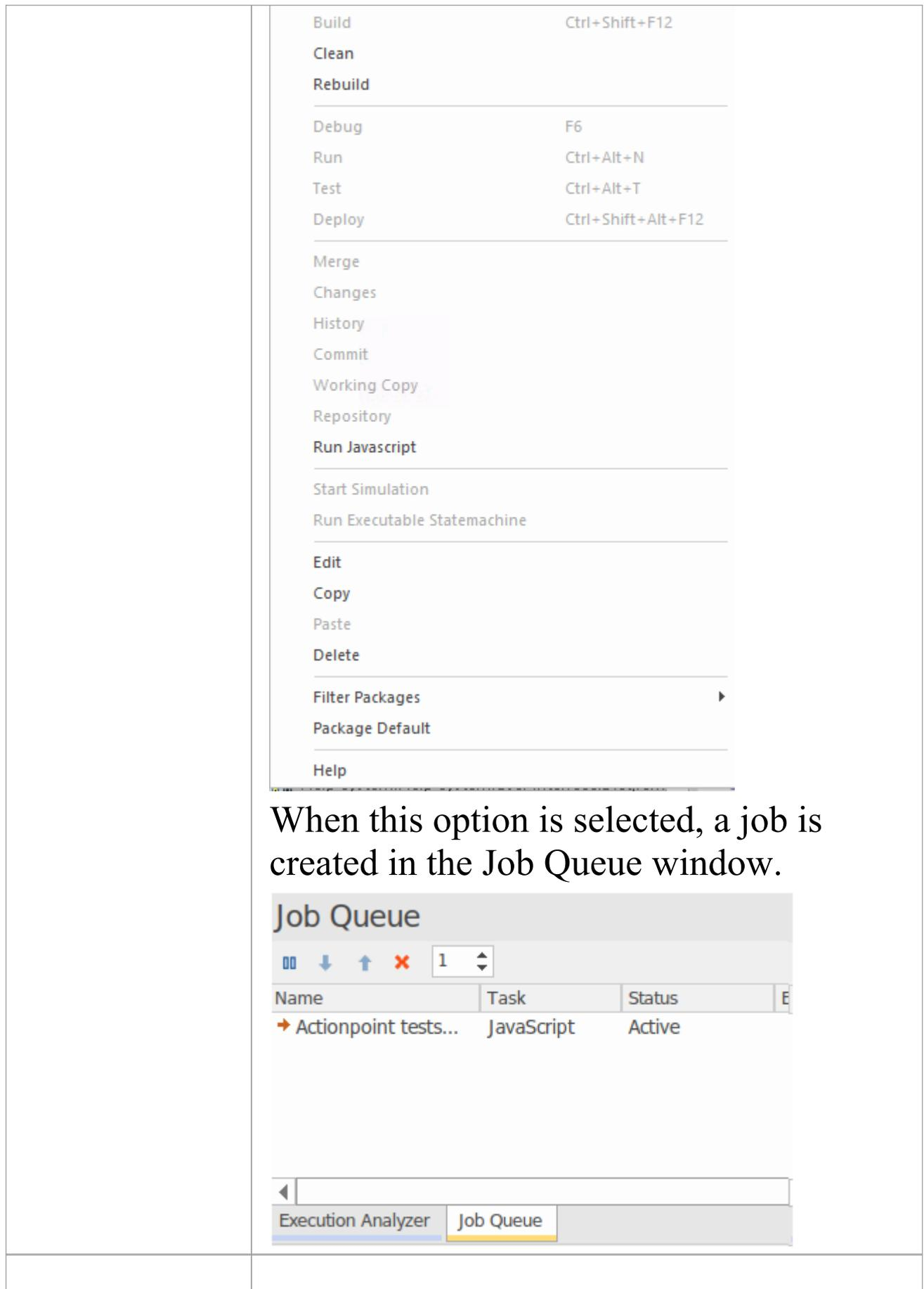
The image shows a software menu with the following items: Build (Ctrl+Shift+F12), Clean, Rebuild, Debug (F6), Run (Ctrl+Alt+N), Test (Ctrl+Alt+T), Deploy (Ctrl+Shift+Alt+F12), Merge, Changes, History, Commit, Working Copy, Repository, Run Javascript, Start Simulation, Run Executable Statemachine, Edit, Copy, Paste, Delete, Filter Packages, Package Default, and Help.
