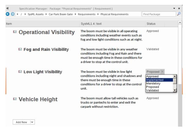
The Specification Manager is the perfect tool for those analysts who are more comfortable working with text rather than diagrams and who are accustomed to working in a Word Processor or Spreadsheet. It has the added advantage that the Requirements are part of a model, and an engineer can trace them to other elements, including Business Drivers, Stakeholders, and Blocks. This image shows that you can specify and manage the Requirement status and other element properties using drop-down lists.
