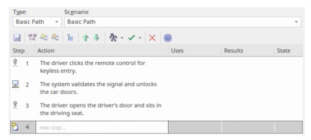
The tool provides a helpful way to generate behavior diagrams such as Activity, Sequence and StateMachine diagrams directly from the scenarios and their steps. These can be synchronized as changes are made to the sequence of steps or to the branch and merge points for alternate and exception scenarios.
