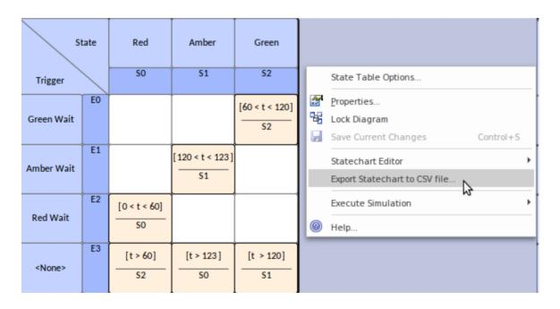
A systems engineer can use state machines to generate executable software code from the model using Executable StateMachines. The code generated is based on its language property. The programming language might be Java, C, C++, C#, or JavaScript; regardless of the language, Enterprise Architect generates the appropriate code immediately ready to build and run.
