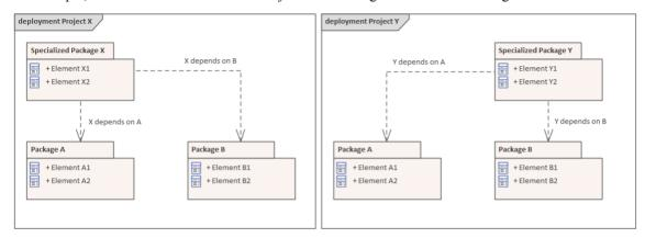
Two common Packages, 'Package A' and 'Package B', are shared across two separate projects, 'Project X' and 'Project Y', through the use of XMI Package files. From the point of view of the common Packages, each of these projects is **'incomplete'**. Project X does not contain 'Specialized Package Y' and similarly, Project Y does not contain 'Specialized Package X'.
