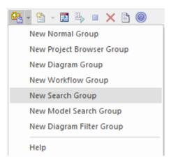
Scripts are managed and contained in groups. Each group has an attribute called 'Type'. This attribute is used to help Enterprise Architect decide how and where the script can be used and from which features it should be made available. The properties of a script group can be viewed from its shortcut menu.
