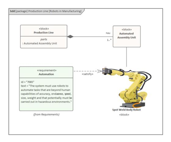
This diagram represents a photograph taken by an engineer of an advanced production line robot assisting with a manufacturing system. The image can be placed into diagrams, and relationships can be drawn between the robot and other parts of the system description, including requirements.
