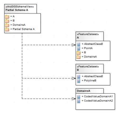
You can also include Packages via indirect Dependency connectors. For example, you can achieve the same result as in the previous example by linking Packages to, say, Feature Dataset A instead of linking them directly to the ArcGIS Schema View.
