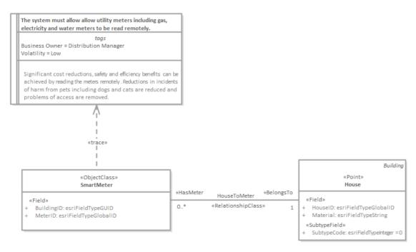
ArcGIS diagram showing a trace between a Smart Meter
