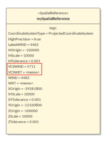
Looking at the WKT Tagged Value in the Tags' tab of the Properties window for this element, you can see that the 'WGS 1984 Australian Centre for Remote Sensing Lambert Projected Coordinate' system has been selected.
