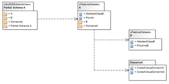
Finally, if you want to create a partial schema that includes only the elements in, say, NestedPackage1, you can model the scenario as a partial schema Package that refers to nested Packages within a Feature Dataset.
