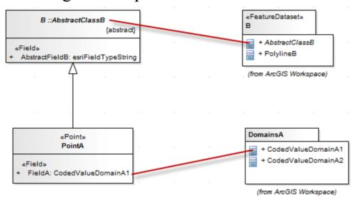
If you wanted to include all CodedValueDomains in DomainsA and all Feature Classes in FeatureDataset B (including any domains they depended on), you could model this situation to include entire Packages of elements in a partial schema via direct and indirect UML Dependency connectors, as shown.
