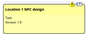
This style displays an icon on the top right corner of the element, representing the element type, with a triangular icon to the left of it representing the priority - red for High
