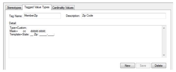
In the diagram, the Mask parameter first defines seven blank spaces, which are occupied by characters defined by the Template parameter.
