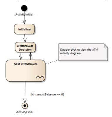
The ATM Withdrawal Activity is a Composite element. If you double-click on it, you open and display the child diagram, which is a more detailed breakdown of the withdrawal process. Similarly, a simulation will open and process the child diagram.
