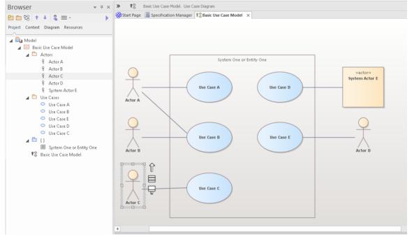
As you can see, there is an underlying model-level element in the Browser window that has a graphical representation in a diagram. Note that you can place a single model element in as many diagrams as you like, and that changing the name or notes or other element properties will be reflected immediately in all diagrams in which the element has been placed.
