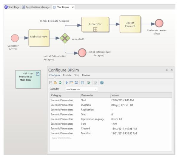
The Configure BPSim window helps you to define several categories of Simulation parameter, each category focusing on one aspect of the Simulation Configuration. For example, you would define:
