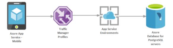
Diagram showing a mobile application using a Smart Phone Traffic Manager and PostgreSQL Database
