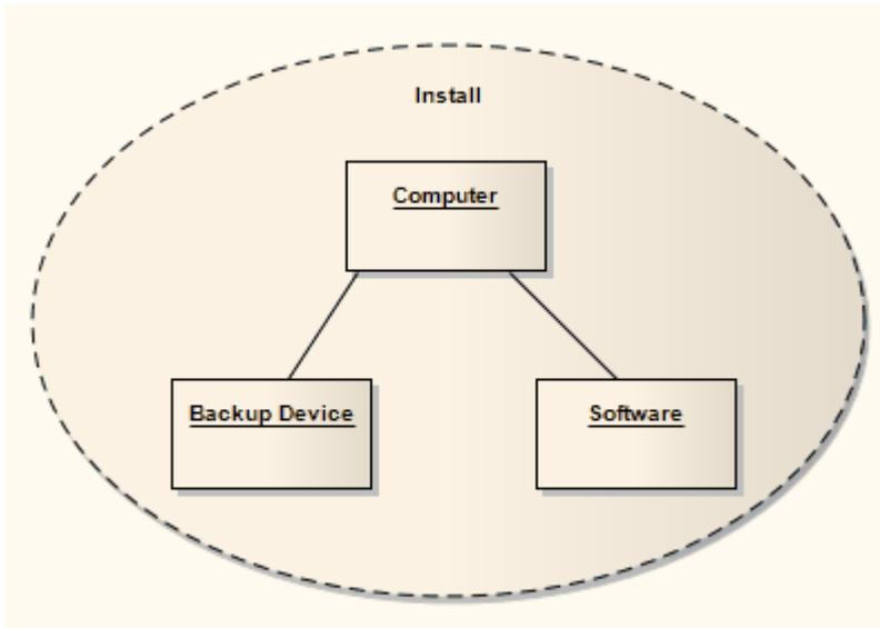
The next diagram uses this Install Collaboration in a Collaboration Use, and applies it to the UtilLoad Class via a «represents» relationship. This indicates that the classifier UtilLoad uses the Collaboration Pattern within its implementation.
