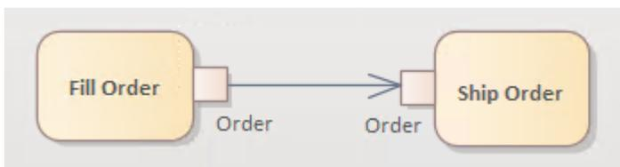
Action Pins can be further characterized as defining exception parameters, streams, or states. Associating a state with a Pin defines the state of input or output values. For instance, the Pin could be called 'Orders', but the state could be 'Validated' or 'Canceled'.
