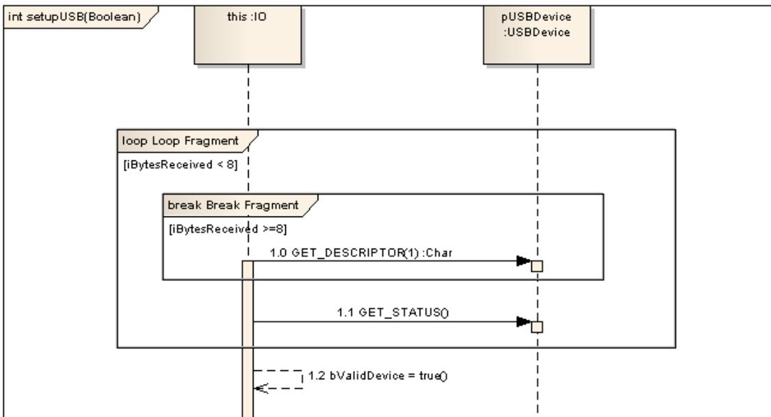
An Interaction element in Enterprise Architect is treated as a behavior of the classifier it is encapsulated within. It can have parameters and return types, which are modeled using the 'Behavior' tab of the Interaction element's 'Properties'
