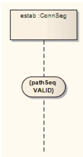
When a State Invariant is moved near to a Lifeline, it snaps to the center. If the sequence object is dragged left or right, the State Invariant moves with it.
