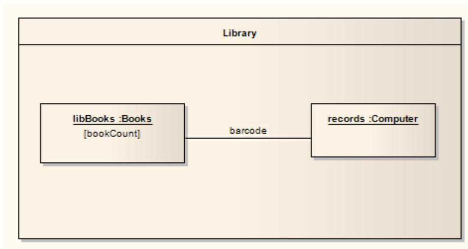
In this diagram there are two Parts, 'libBooks' and 'records', which are instances corresponding to the Classes 'Books' and 'Computer' respectively. The relationship between the two Parts is indicated by the connector, reflecting that communication between the Parts is via the barcode. This contained structure and its Parts are properties owned by the Library Class.
