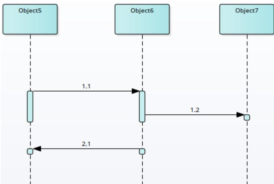
Message 1.1 passes from Object 5 to Object 6, and then Message 1.2 passes to Object 7 and Message 2.1 passes back to Object 5. It appears that the Messages go in the
