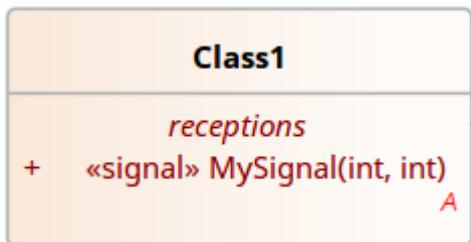
A Reception cannot be created without a Signal element, which either already exists or is created as a step in creating the Reception. The name of the Reception is drawn from the name of the Signal element, and the attributes of the Signal define the parameters of the Reception. Any changes to the Signal are reflected in the Reception, and vice versa.
