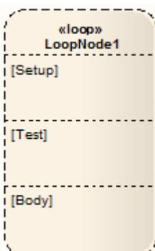
You define the Loop nodes by dragging Action elements from the Diagram Toolbox page into the 'Setup', 'Test' and 'Body' partitions. The 'Body' partition can contain several
