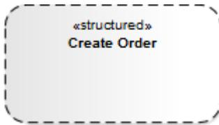
You can nest other elements underneath the Structured Node, including other Structured Activity elements such as Conditional, Loop and other Structured Node elements.
