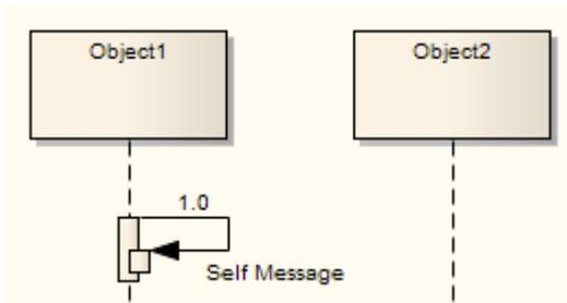
A Self-Message reflects a new process or method invoked within the calling lifeline's operation. It is a specification of a Message, typically in a Sequence diagram.
