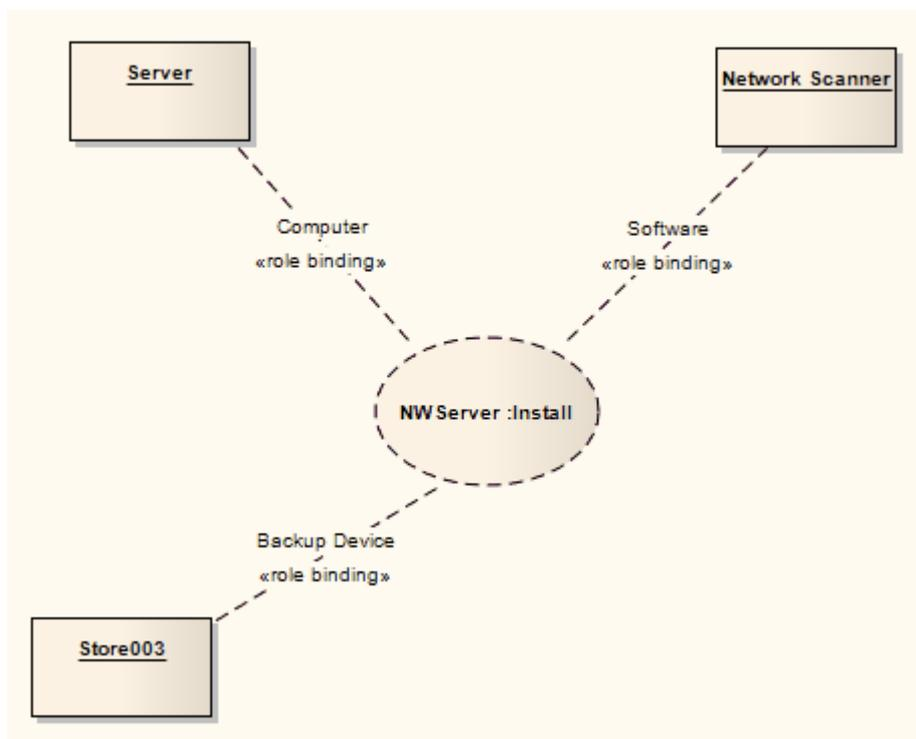
To create a Collaboration Use, drag the icon from the 'Composite' page of the Diagram Toolbox onto the diagram.
