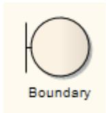
A Boundary is a stereotyped Object that models some system boundary, typically a user interface screen. You can also create a Boundary as a stereotyped Class. Boundary elements are used in analysis to capture user interactions, screen flows and element interactions (or 'collaborations').
