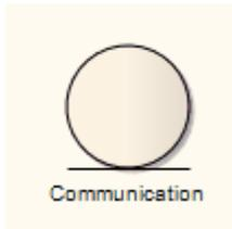
An Entity is a stereotyped Object that models a store or persistence mechanism that captures the information or knowledge in a system. It is the Model in the Model-View-Controller Pattern.
