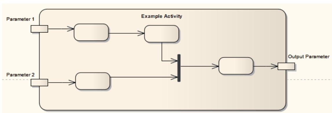
You can define an Activity as a composite element, either during creation or during later edits. When creating a composite Activity element, it is simpler to apply the mechanism for creating Structured Activity elements, which
