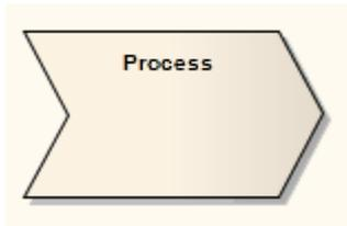
A Process is an Activity element with the stereotype process, which expresses the concept of a business process. Typically this involves inputs, outputs, workflow, goals and connections with other Processes. The Process element is typically used in Analysis diagrams.
