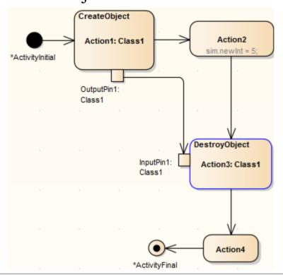
Perform a Simulation on the diagram. The process passes the Object name or value into the Input Action Pin as a parameter. When the DestroyObject Action is executed, it deletes the Object having that name or value from the model.
