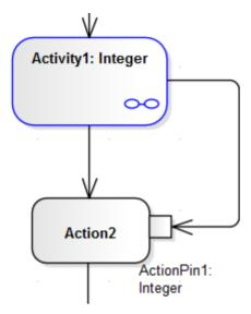
You can simulate this by setting a simple JavaScript statement to set the return value in the Activity's child element (such as this.return=12;) and, running the simulation, see the value transferred to the Action Pin in the Locals window.
