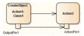
Perform a Simulation on the diagram. When the CreateObject Action is executed, it creates an Object having the properties of the classifier, and stores it in its Output Pin. The Object itself is passed through the Object Flow connection to the Input Pin of Action 2, where its properties can be listed in the Locals window for the Simulation.
