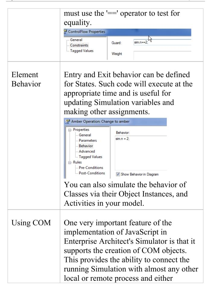
influence the Simulation based on external data, or potentially change data or behavior in the external world based on the current Simulation state (for example, update a mechanical model or software Simulation external to Enterprise Architect). The syntax for creating COM objects is shown here:
