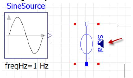
Similarly for Simulink, this is the resulting model showing the lack of a connector from the SineOutput:
