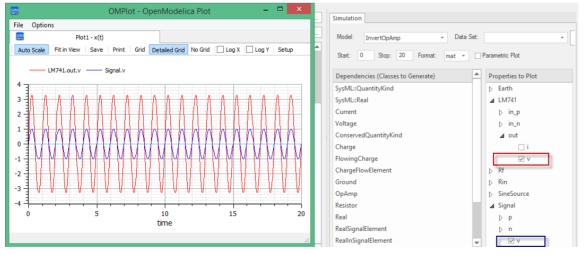
In the legend you can see LM741.out.v and 'Signal.v that are plotted, and match them with the two properties selected under *Properties to Plot*.
