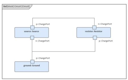
Notice that this follows the same structure as the original circuit diagram, but the symbols for each component have been replaced with properties typed by the Blocks we have defined.
