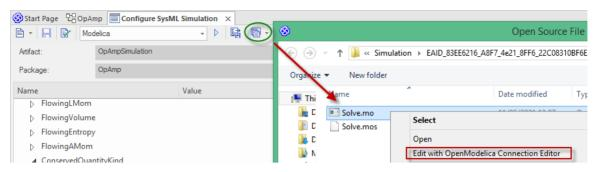
When opening the generated model in Modelica, using the icon on the Toolbar, this is the view showing that the connector is not linked to the triangle that is the import to the Signal object:
