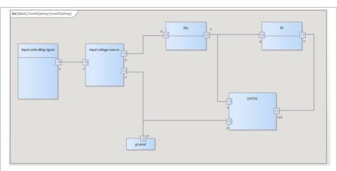
Notice that this follows the same structure as the original circuit diagram, but the symbols for each component have been replaced with properties typed by the Blocks we have defined.
