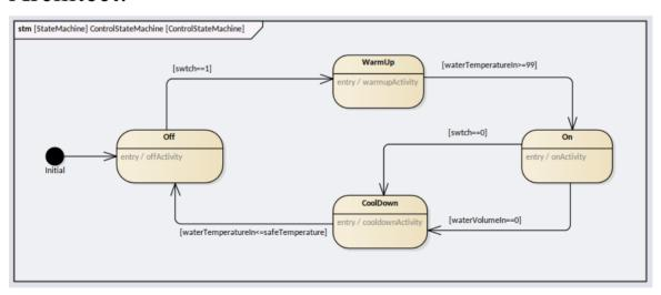
This is an example of how the code generated by Enterprise Architect, from the diagram above, is rendered as a Stateflow diagram:
