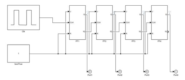
The circuit in this example includes a pulsed digital signal source, four Flip-Flops and a logical Boolean true state to form a simple frequency divider circuit.
