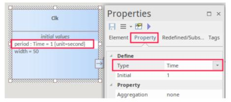
The J & K Ports require a fixed logical 'True' state. This is defined using a Table set to 'true' using an initial value, as shown here for Modelica.
