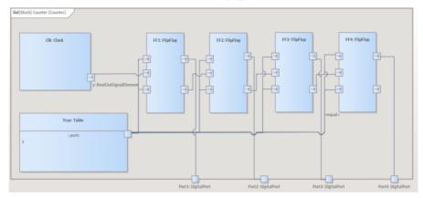
Notice that this follows the same structure as the original circuit diagram, but the symbols for each component have been replaced with properties typed by the Blocks we have defined.
