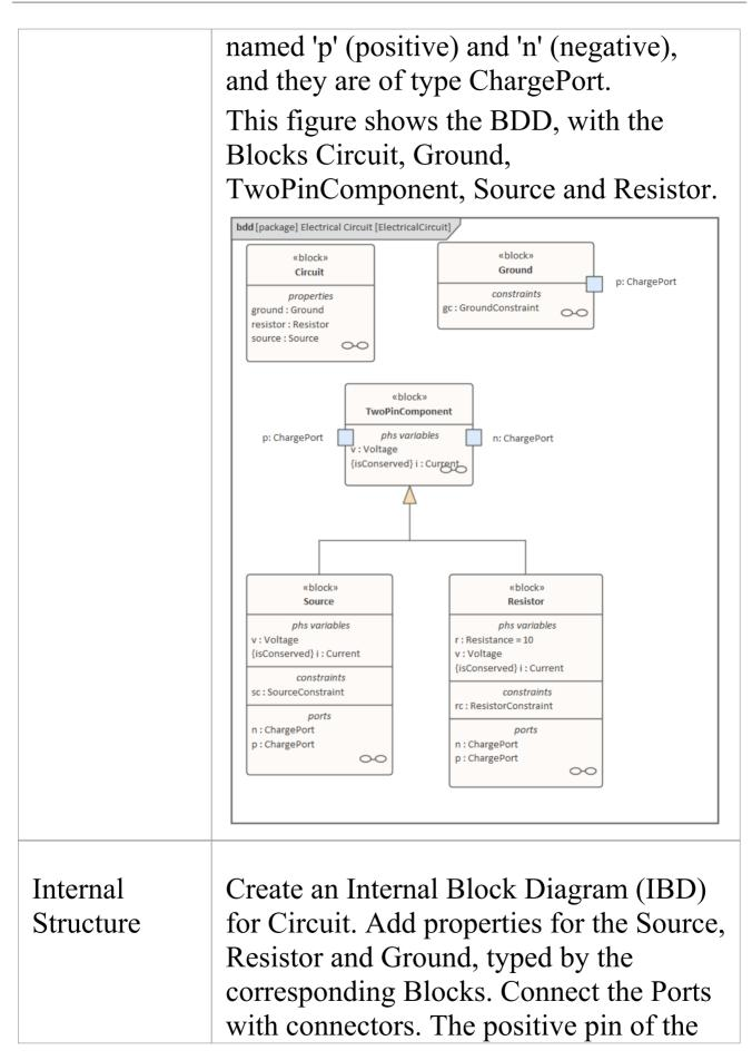
Source is connected to the negative pin of the Resistor. The positive pin of the Resistor is connected to the negative pin of the Source. The Ground is also connected to the negative pin of the Source.
