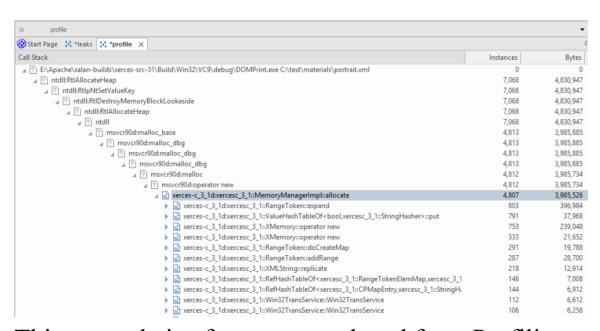
This example is of a report produced from Profiling a demonstration program in the Xerces project from Apache. The program iterates over the Document Object Model (DOM) for a provided XML file.
