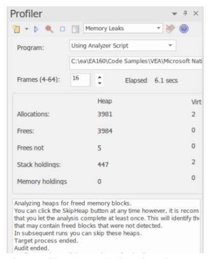
The Profiler control, showing the count of memory allocations and the count of operations that are memory free.
