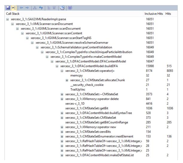
This detailed report shows the unique set of Call Stacks/behaviors as a weighted Call Graph. The weight of each branch is depicted by a hit count, which is the total hits of that branch plus all branches from this point. By following the hit trail, you can quickly identify the areas of
