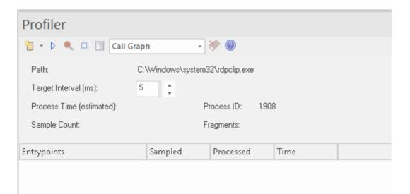
The Profiler is controlled using its toolbar buttons. Here you can attach the Profiler to an existing process (or JVM), or launch the application for the active Analyzer Script. The Profiler window displays the details of the target process as it is profiled. These details provide feedback, letting you see the number of samples taken. You also have options for
