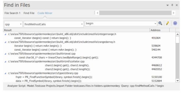
The currently active Analyzer Script, and also the query parameters, are indicated across the bottom of the 'Code Miner' page of the search tool.
