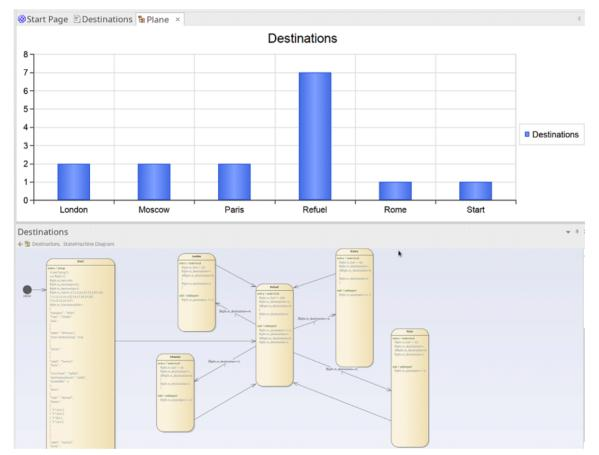
In addition to Charts you specifically produce, a summary Chart can be produced automatically by a simulation. All that is required is adding a DynamicChart Artifact to the Package and giving it the same name as the StateMachine. The default Chart summarizes the State transitions taken during execution of a simulation. If a default Chart is found when the simulation completes, that Chart's data is updated, and displayed automatically.
