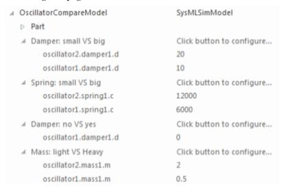
On the 'Simulation' page, select 'OscillatorCompareModel', plot for 'oscillator1.mass1.s' and 'oscillator2.mass1.s', then choose one of the created datasets and run the simulation.
