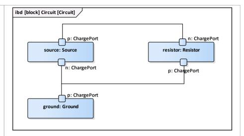
Notice that this follows the same structure as the original circuit diagram, but the symbols for each component have been replaced with properties typed by the Blocks we have defined.
