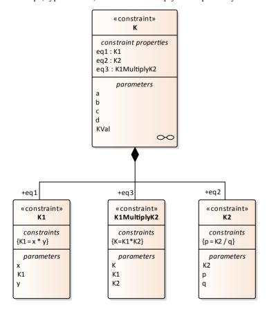
Create a Parametric diagram in Constraint Block 'K' and connect the parameters to the constraint properties with Binding
