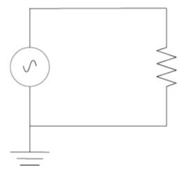
The circuit includes an AC power source, a ground and a resistor, connected to each other by wires.
